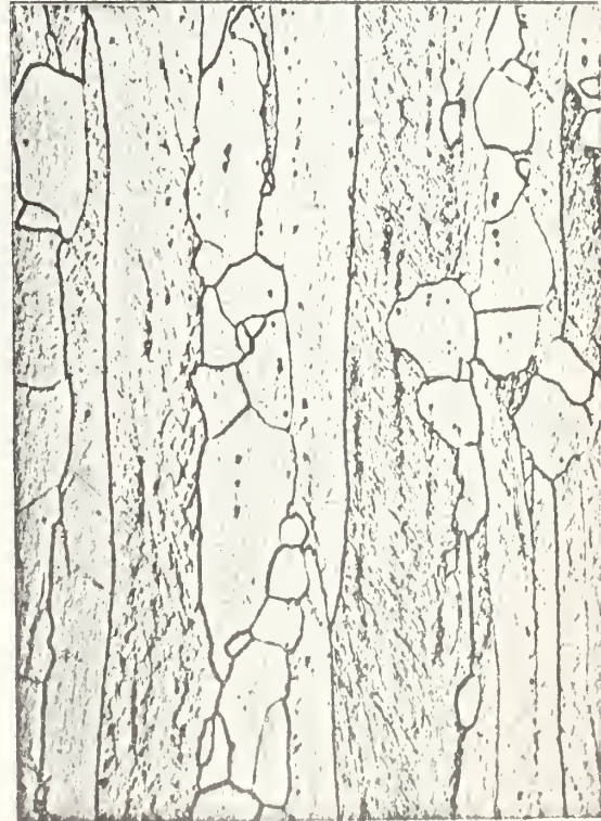
FIG. 30 AT 482°C FOR 11.7 HOURS (ROCKWELL 30T 62.7)
